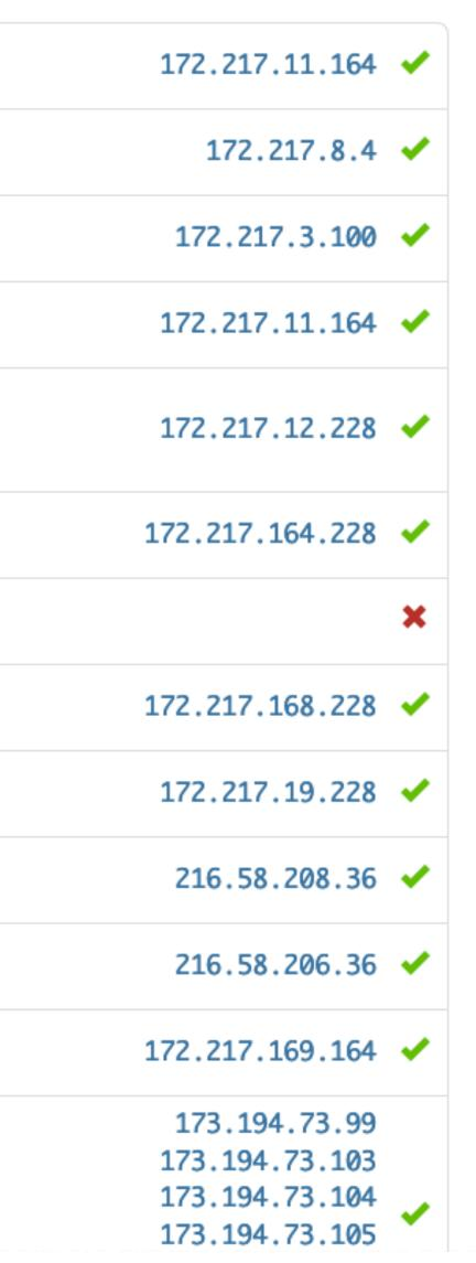
DNS servers can respond with the IP for the load balancer that is closest to the client **Reduces connection** latency and helps to distribute traffic Doesn't fix availability... If local datacenter goes
