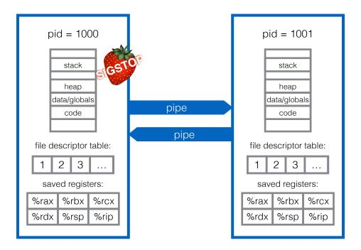
Processes can synchronize using signals and pipes
